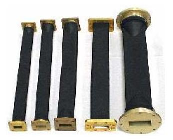
Actox stocks several styles of twistable/flexible waveguide for immediate delivery. These flexible assemblies are used to isolate vibration and to eliminate installation difficulties caused by misalignment of rigid sections. Actox supplies two basic types of flexible waveguide. Type "TF" is more common of the two types. "TF" is a twistable and flexible waveguide which can be twisted or flexed into extreme conditions.
